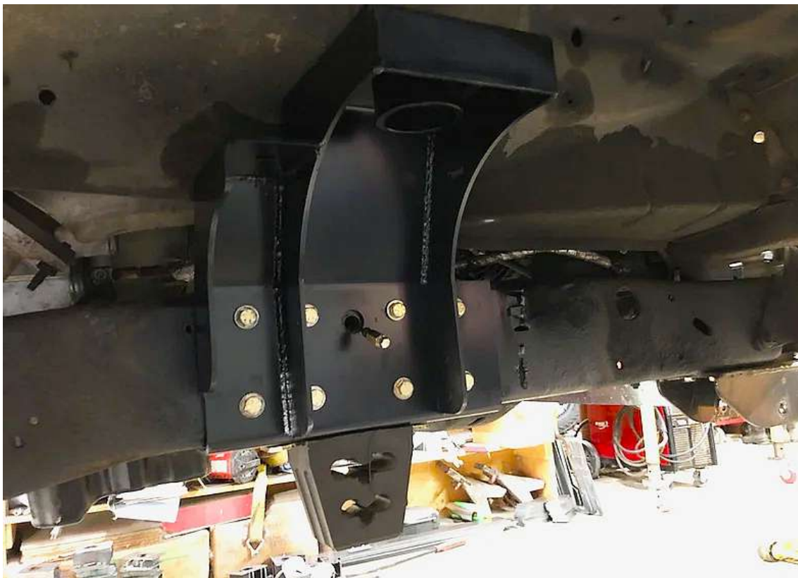
SD brake hoses bolt to buckets here on forward side. 05-07 brake hose shown
