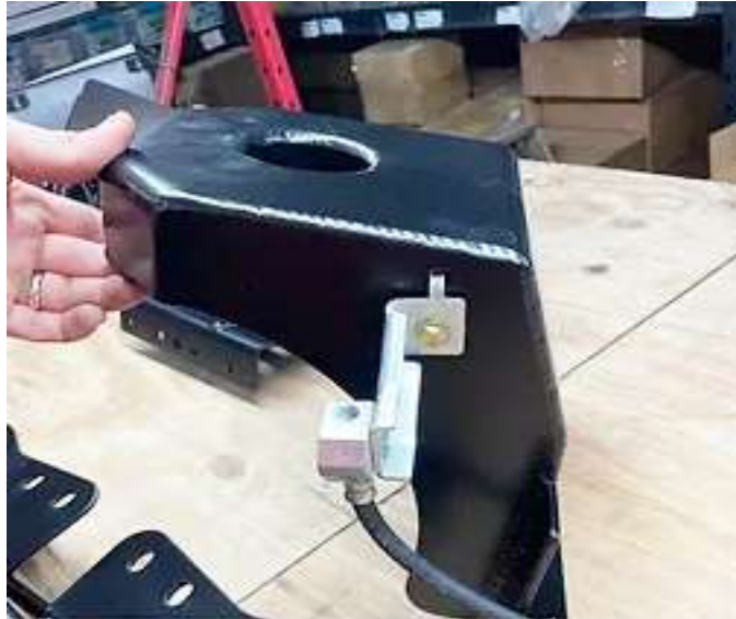
SD brake hoses bolt to buckets here on forward side. 05-07 brake hose shown
