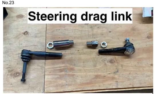
Use 2005-new SD tie rod end at passenger side knuckle and new BBB supplied tie rod end at pitman arm, and weld machined ends in F03 hardware bag to a lengh of 1.0" ID 1.5" OD DOM tube
