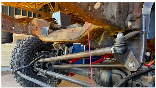
Point pitman arm straight forward, straighten tires as much as possible, and measure overall length of drag link. Keep in mind length of weld on ends and jam nuts before cutting.
