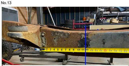
All radius arm brackes, 4 link brackets, and drilling templates will have one slotted hole on their forward side that is intended to locate on this hole in your frame about 11.5" back from the rear flange of your forward cab mount
